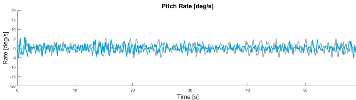
Performance results are measured with the system on and off as a reduction of standard deviation in pitch and roll rates at all frequencies at a constant heading and speed.
