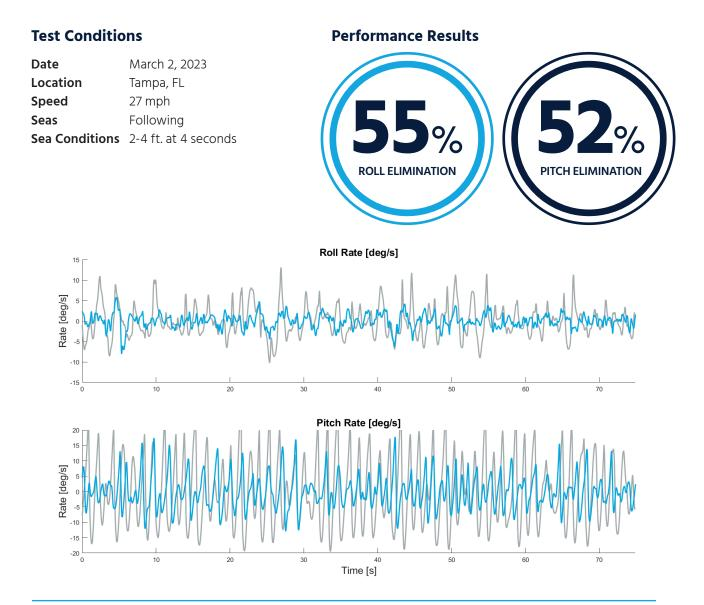
Performance results are measured with the system on and off as a reduction of standard deviation in pitch and roll rates at all frequencies at a constant heading and speed.
